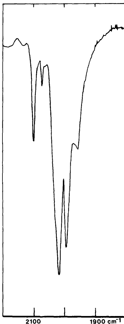
FIG. 5. Infrared spectrum of solution obtained from Pr 3 PO, Ru 3 (CO) 12 , and HI, after catalysis. 75 ml Pr 3 PO, 6 mmol Ru, 6 mmol HI. Conditions of reaction: 86.1 MPa, H 2 :CO = 1, 230°C. Band at 2100 cm -1 and shoulder at 2030 cm -1 are assigned to [Ru(CO) 3 I 3 ] - .
